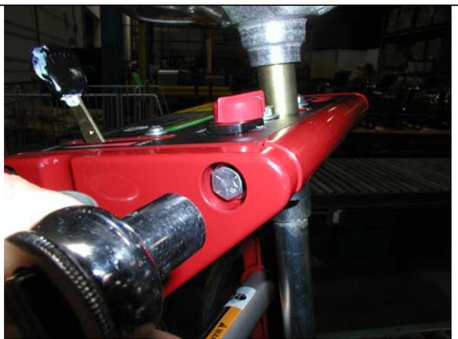
6. Remove bolt from forward end of control panel on right side of saw.
