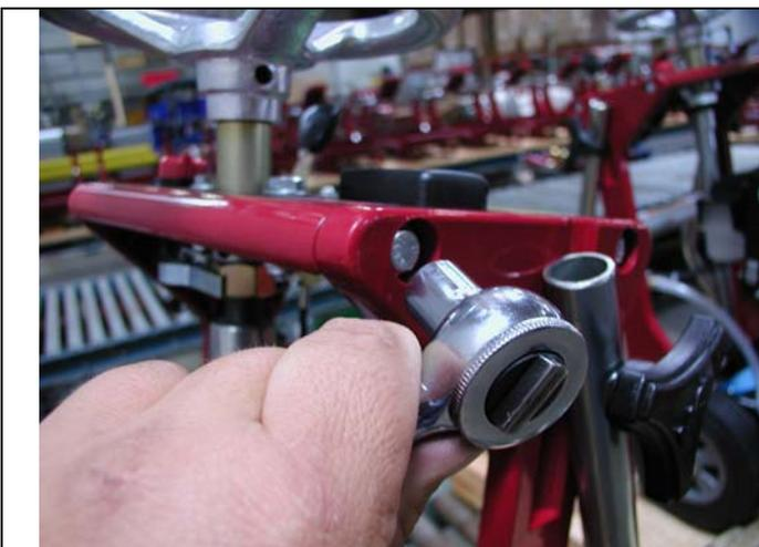
5. Remove bolt from forward end of control panel on left side of saw.
