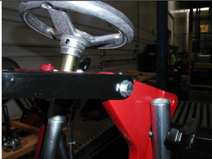
9. Using screw (#4), washer (#3), lock washer (#2) and nut (#1), attach upper tabs of lifting bail to forward holes in casting and control panel.
