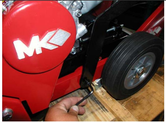
8. Again using flat head screw (#7) and spacer (#6), screw right lower leg of lifting bail (#5) through casting into tubing.
