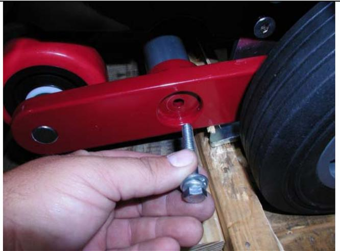
2. Remove tube bolt in front of left wheel.
