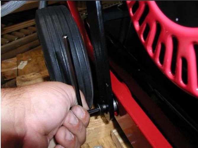
7. Put lifting bail (Item #5) in position, and using flat head screw (#7) and spacer (#6), screw lower right leg through casting into tubing.
