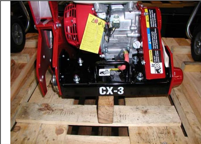
1. Insert block under front of saw frame.
