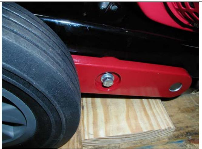
4. Remove tube bolt in front of right wheel.
