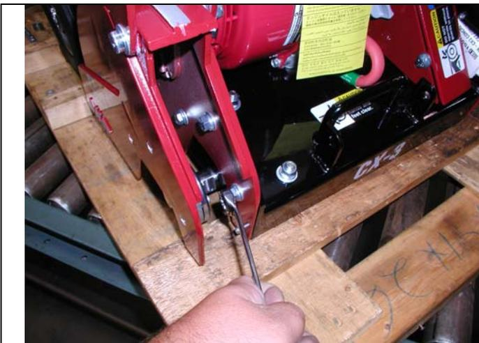
3. Remove blade guard by removing 3 bolts from inside of guard.
